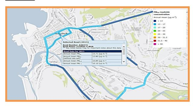
At Terrace Road (indicated by arrow from text-box on map above) the modelled concentration as an annual mean in 2015 was  $15.71\mu g/m^3$  (12.8 without sea salt). This concentration, again at a "worst, roadside and hot-spot location" in Ceredigion, is well below the annual PM10 standard of  $40\mu g/m^3$ .
