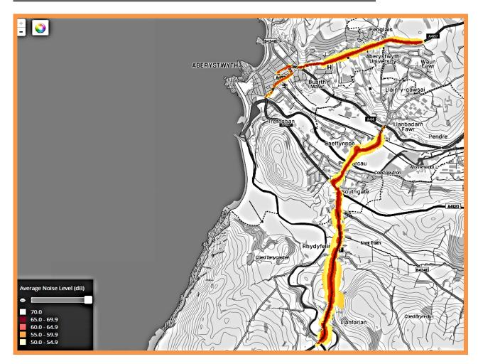
AVERAGE, roadside, <u>night time</u> noise levels (in dB) on the roads in and approaching Aberystwyth in the map displayed above are estimated to vary between 50 and 60dB. These ESTIMATES are above the 40dB (and possibly the 55dB interim) guideline levels for night time noise recommended by the World Health Organisation.
