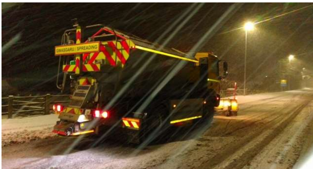
Figure 14 – An 18 tonne designated gritter keeping the roads open.
