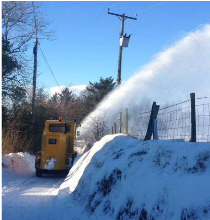
Figure 15 – A Rolba snowblower in action, snowblowers are used in extreme conditions to clear snow.
