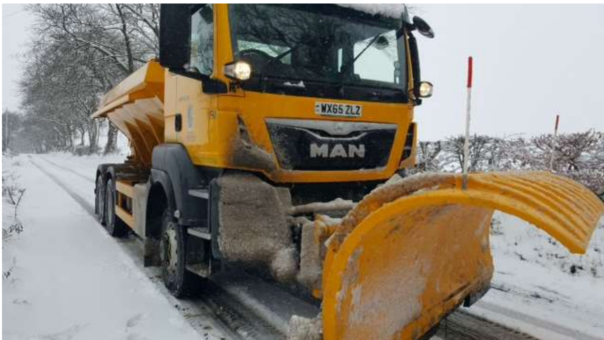
Figure 5 – Designated 26t tonne MAN gritter in action.
